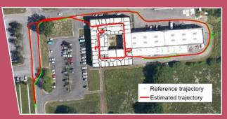
1 km walk on two floors. Inertial sensor, magnetometer and GNSS Rx. Accuracy: 0.3% of the traveled distance (state of the art: 1-2%)
